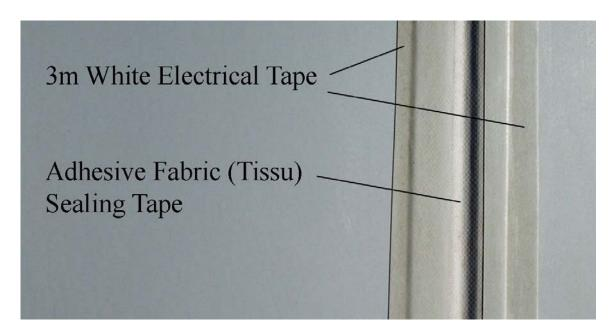
The tape is applied with the control surface fully deflected. (In the case of the gear doors, with them closed.) The excess fabric is tucked into the gap as the control surface is returned to the neutral position.
